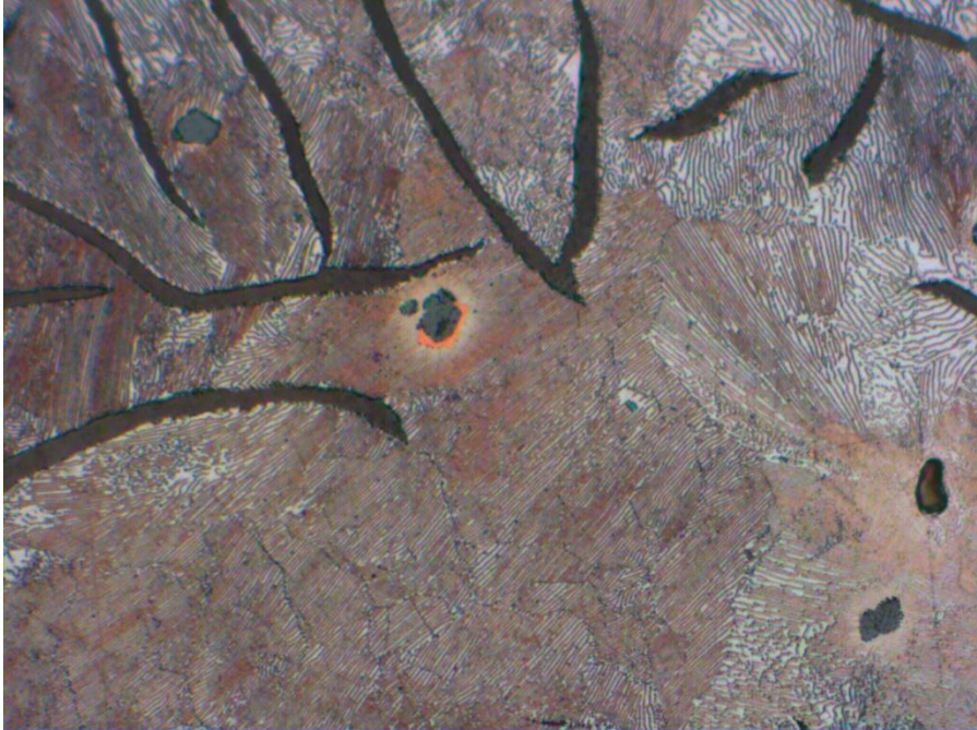
Figure 4-31: In the middle of the image, a Ti(C,N)-inclusion nucleated to a manganese sulfide.
