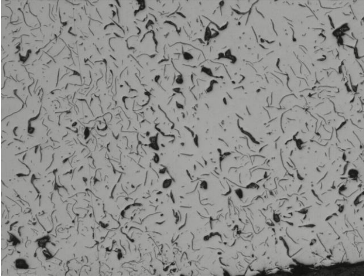
Figure 4-9: Graphite structure of the top area in the bulk material of engine block 3. This sample have distribution type D, which is recognized by the way the graphite flakes are orientated.
