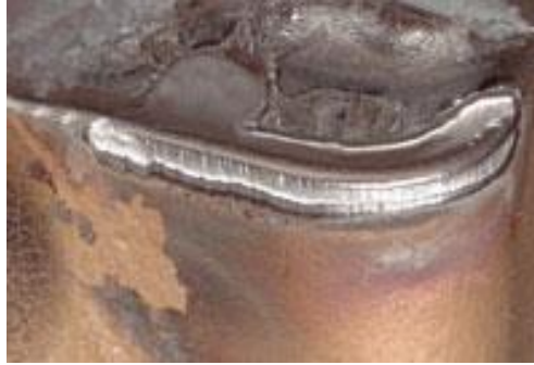
Figure 2-8: Typical appearance of flank wear on a cutting edge [21].
