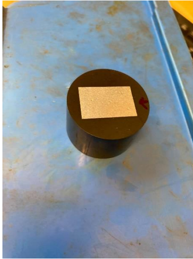
Figure 3-4: Material sample mounted in epoxy.
