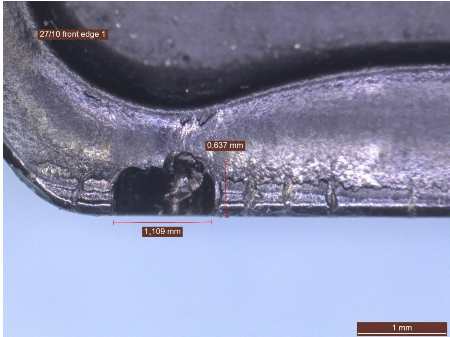
Figure 4-22: A cutting insert with a large chunk of edge torn out.
