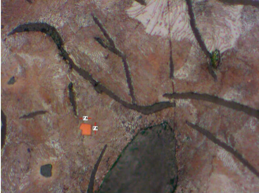
Figure 4-29: The orange square shaped object is a large Ti(C,N)-inclusion with sharp edges. The curved strings are graphite flakes and the large black object in the lower middle is a manganese sulfide inclusion
