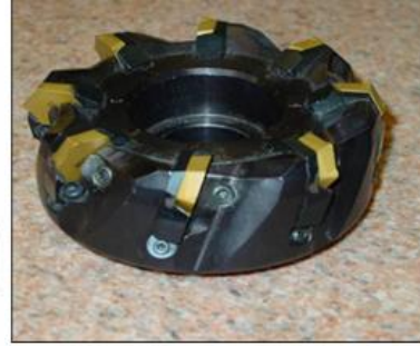
Figure 2-3: To the left, a schematic illustration of a milling head. To the right, a picture of a milling head [20].
