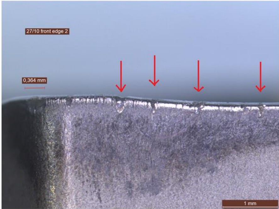
Figure 4-21: Initiated thermal cracks. Red arrows indicates the small, periodical notches typical for thermal cracks.
