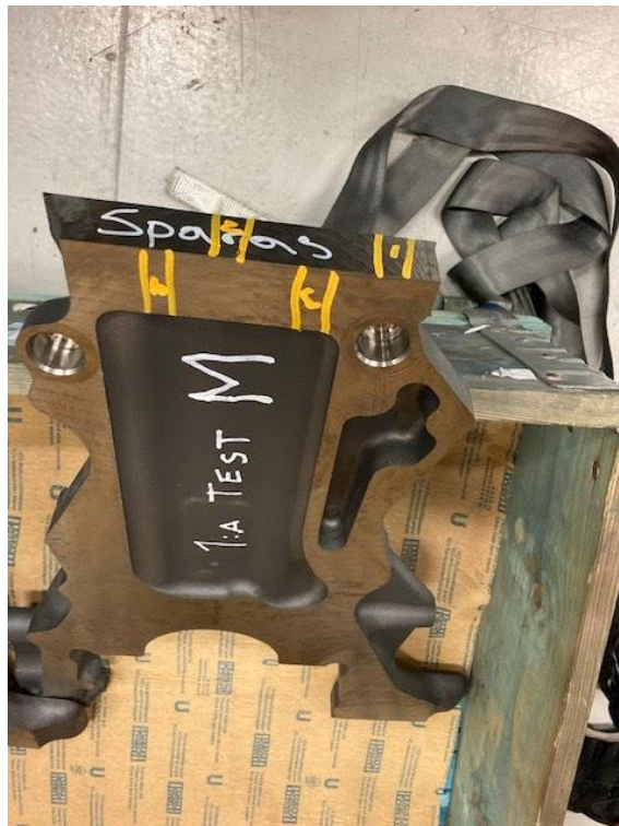
Figure 3-3: Sawed of gable used in a destructive test. The yellow markings indicate where the material sample were taken in engine block 1 and 2.
