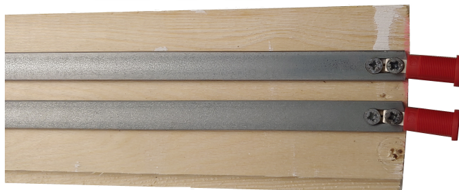
Figure 3.8 Home made light rail.
