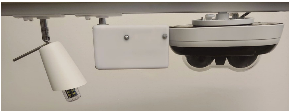
Figure 4.4 Fully setup prototype on light rail with lamp and camera.
