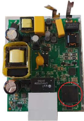
Figure 3.15 Deconstructed TL-PA4010, PCB layout, PHY highlighted.
