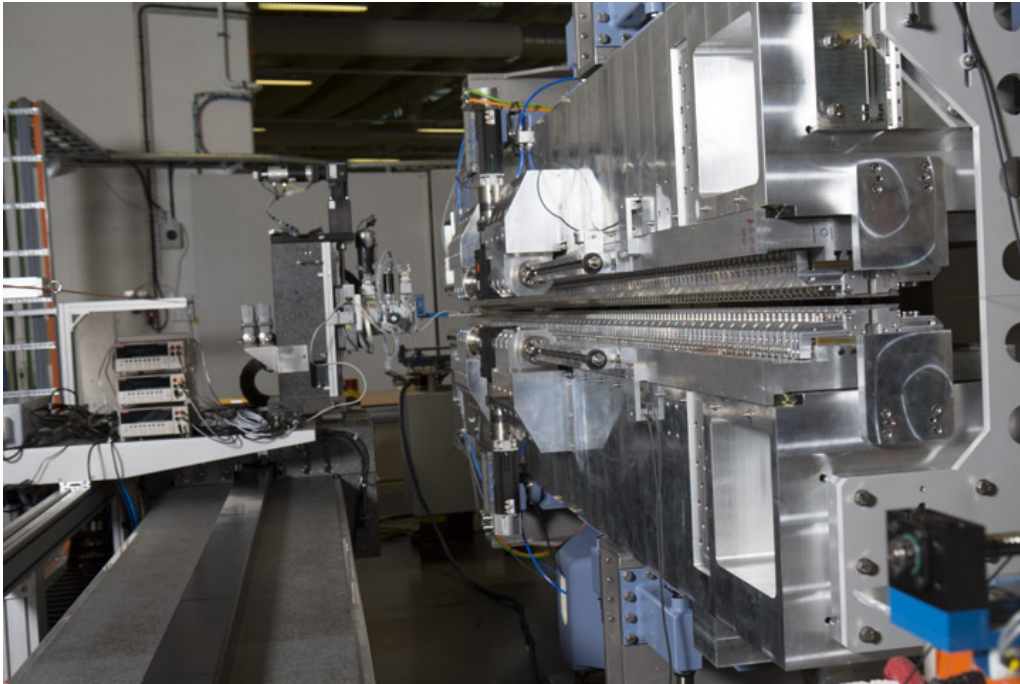
Figure 93: MAX IV Hall-probe mapper (left) scanning an Undulator (right).
