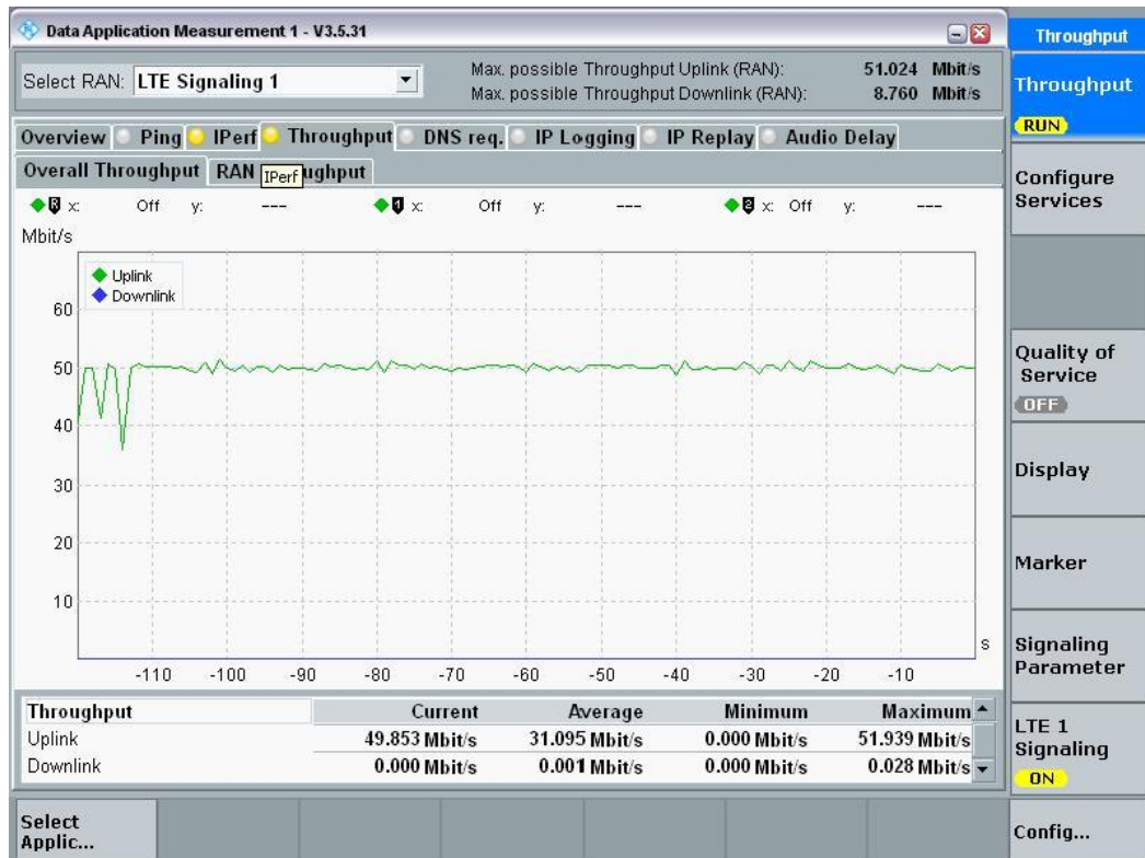
Figure 15: Screenshot of the screen of CMW500 displaying throughput when connected to the DUT
