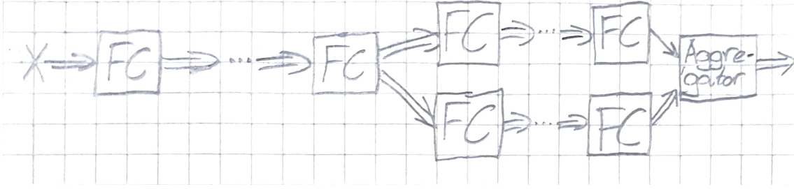
Figure 4.3: The Dueling DQN architecture.
