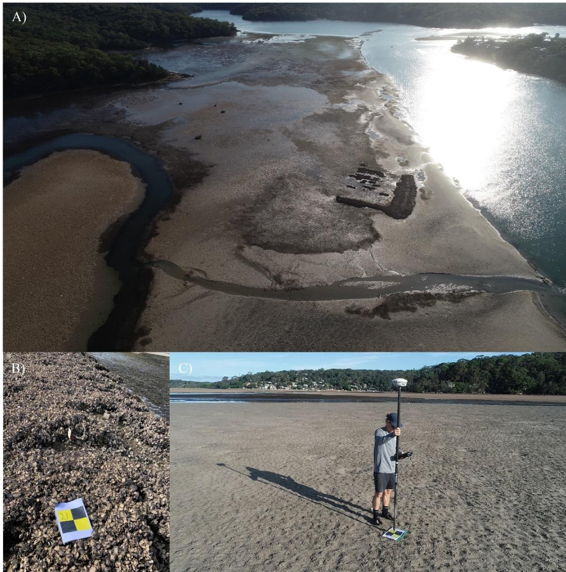
Figure 4.6. Field work photos taken during the drone survey. A) Aerial image of the Port Hacking Reef taken from 120m altitude looking away from the estuary opening towards the West-Southwest. B) GCP marker #21 placed on top of the reef. C) Measuring coordinates of GCP markers using the RTK-GNSS on the sediment substrate surrounding the reef.
