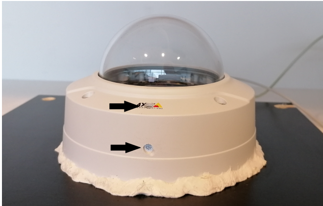
Figure 4.1: The dome camera with two microphones. The arrows marks the placement of the microphones.
