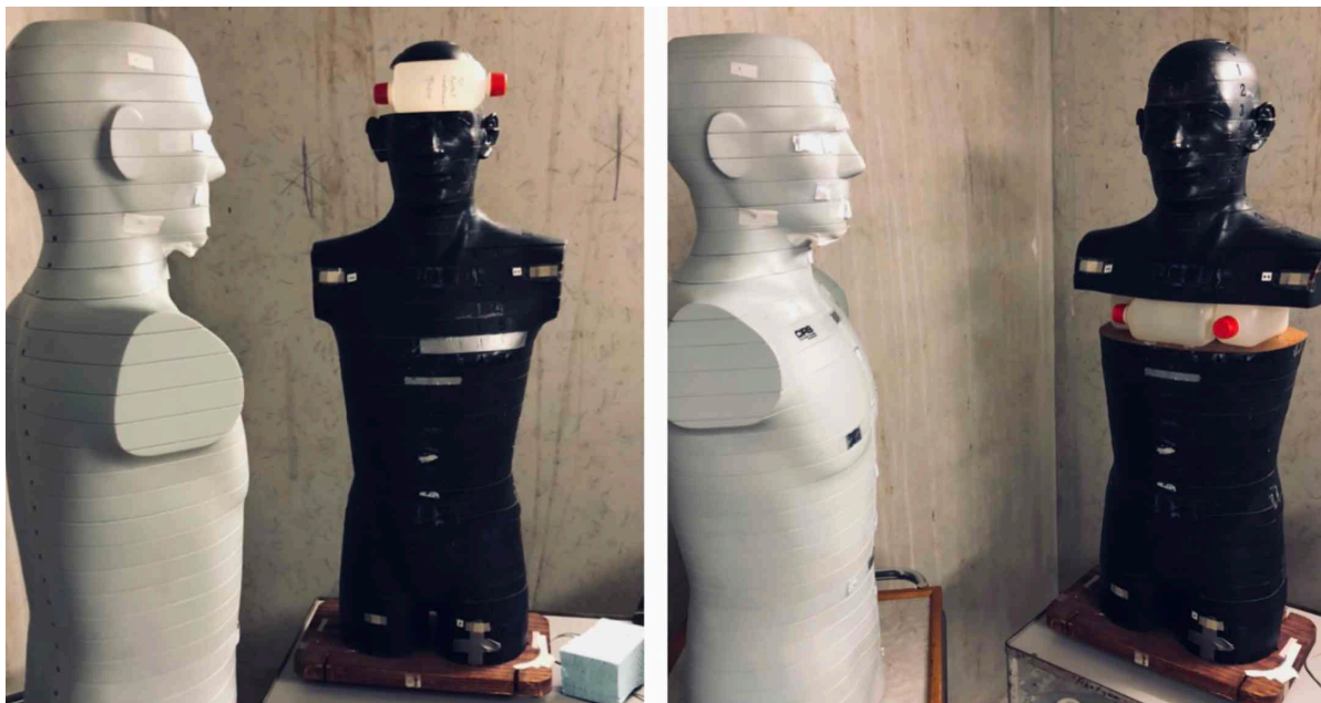
Figure 10: Experimental Setup 3 and 4 for the simulation of radiopharmaceutical distribution of ^{137}\text{Cs} in the brain (left) and in the torso (right). The light phantom (CIRS ATOM) represents the staff member and the dark phantom (RANDO) represents the injected patient.
