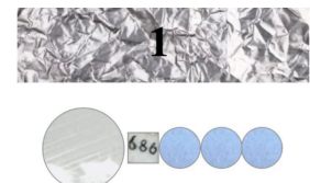
Figure 4: Dosimeter kit in row geometry for 1 Al 2 O 3 , 1 LiF and 3 NaCl pellets.
