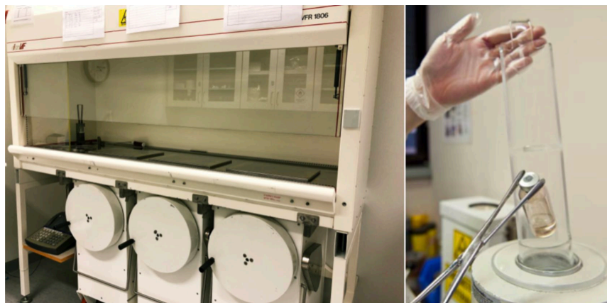
Figure 2: The ^{99m}\text{Tc} elution is prepared with the ^{99}\text{Mo} -generator (left image) and the activity is measured with the ion chamber (right image, Bailey et al, 2015).
