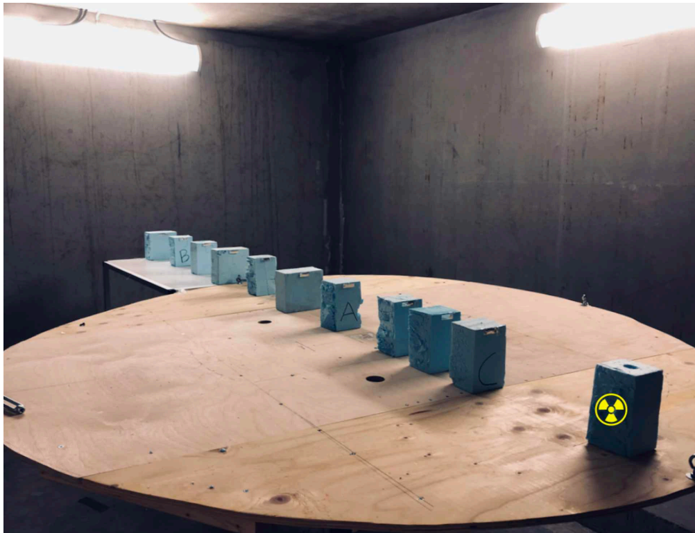
Figure 6: Experimental setup for the dose rate measurement. The radiation source is placed in the center of one styrofoam block, placed at one end of the table and the dosimeter kits were attached to the other 10 blocks at different distances from the radiation source.
