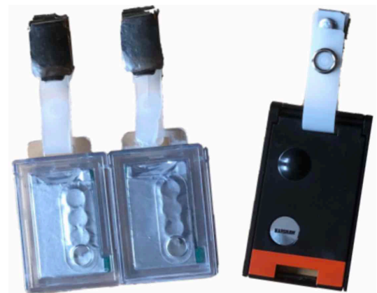
Figure 12: Left figure shows self-made dosimeters containing all three detector materials (1 Al 2 O 3 , 1 LiF, 3 NaCl pellets). Right figure shows commercially available TLD worn by medical staff.
