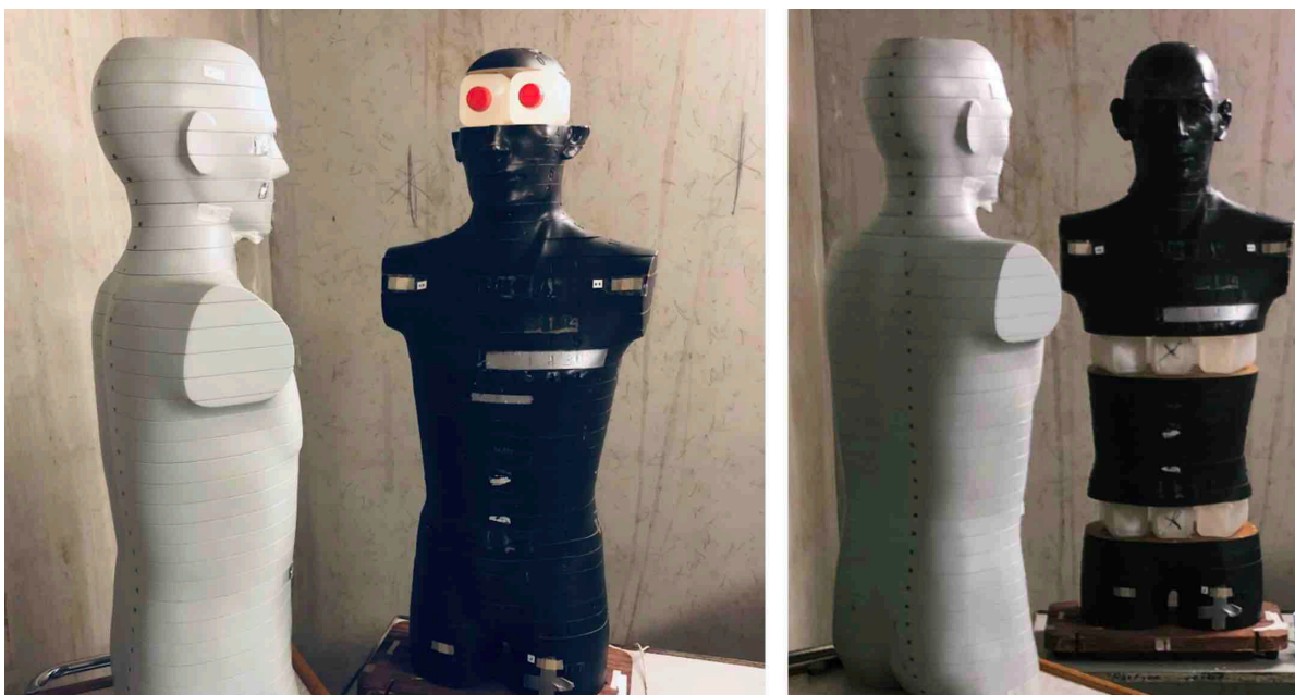
Figure 9: Experimental Setup 1 and 2 for the simulation of radiopharmaceutical distribution of ^{99m}\text{Tc} in the brain (left) and torso (right). The light phantom (CIRS ATOM) represents the staff member and the dark phantom (RANDO) represents the injected patient.
