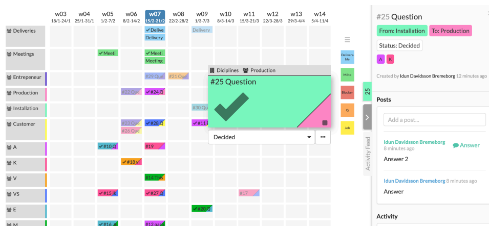
Figure 1.1: An example from a Yolean board showing a question and the answer.
