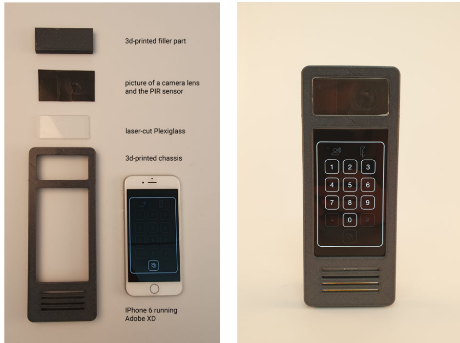
(a) The prototype Barbro before assembly (b) The prototype Barbro after assembly
