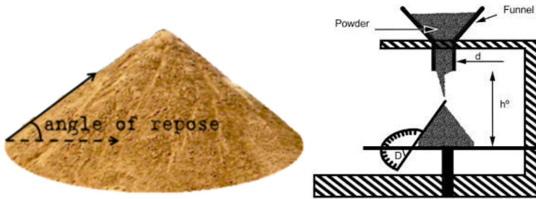
Figure 2 The angle measured in angle of repose tests, as well as a schematic view of an angle of repose measurement with an open base and fixed height. [A][D]
