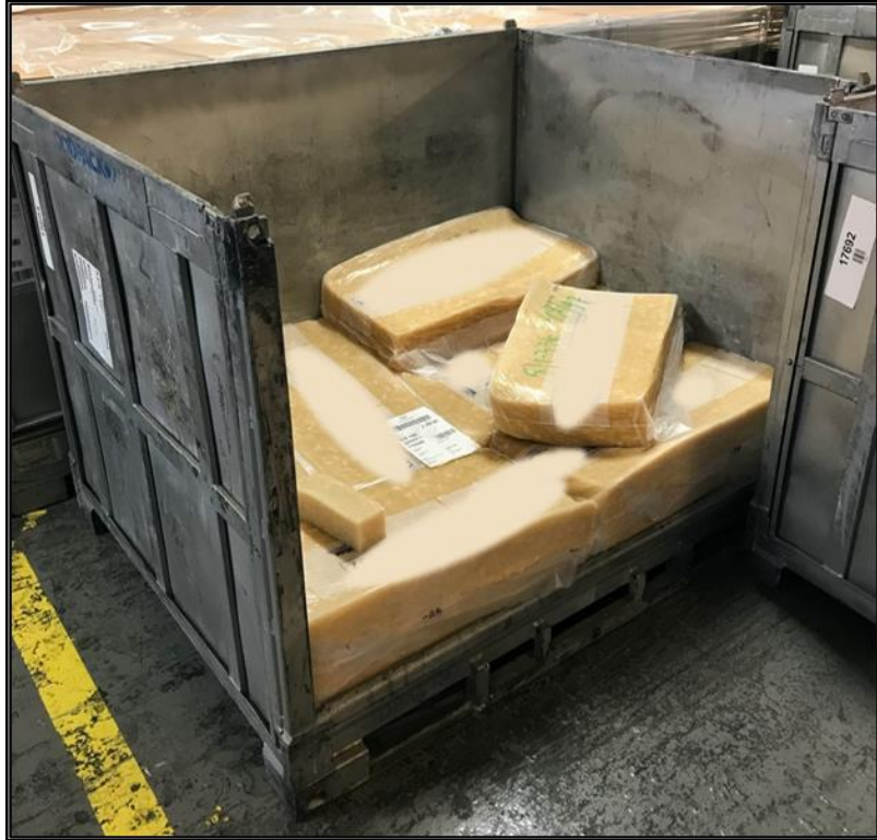
Figure 4: The polymer bins in which polymer is delivered from the suppliers
