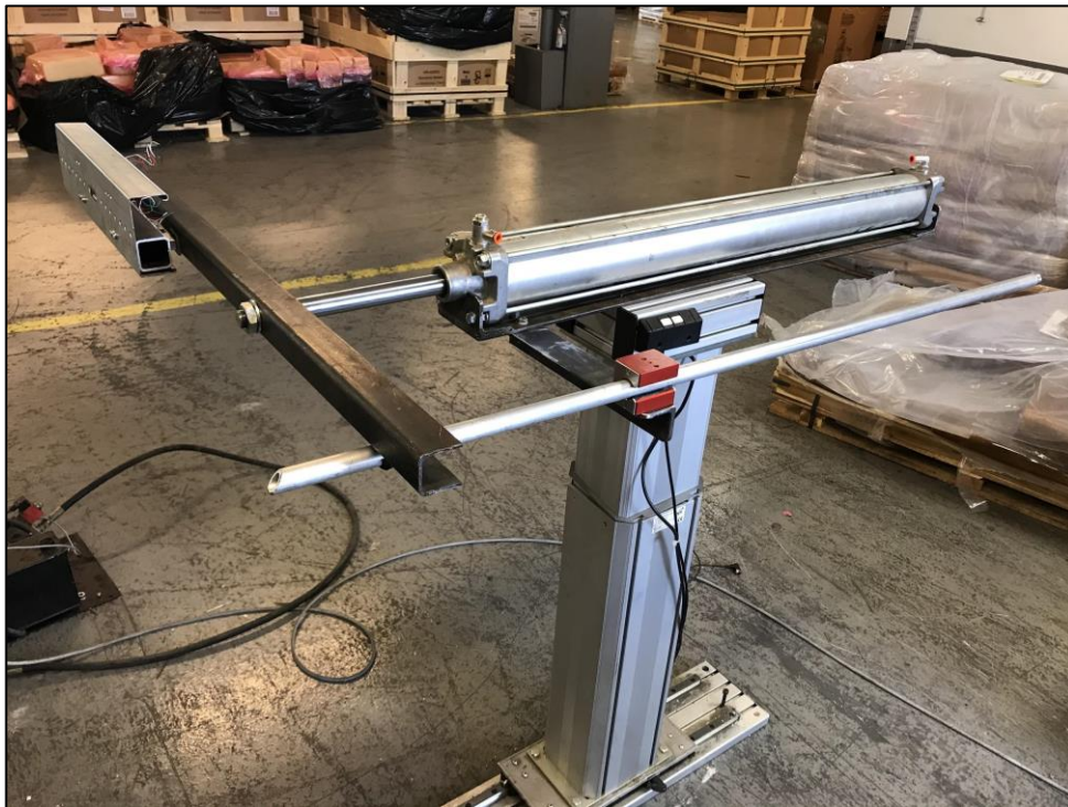
Figure 27: The piston mounted on a small lifting table, with a guiding rod for stability
