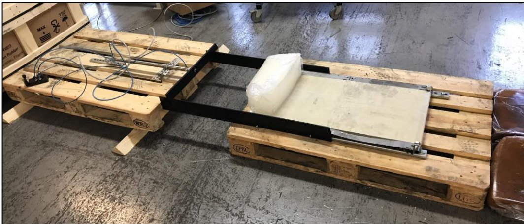
Figure 24: Initial prototype, used for testing if a piston could push a piece of polymer
