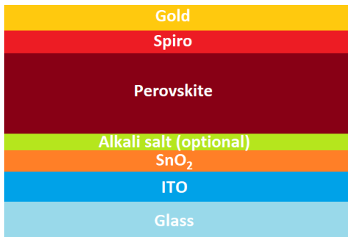
Figure 3.1: The solar cell stack, with the front side of the solar cell at the bottom in the figure. The alkali salt layer is only included for batches 3-4.
