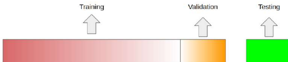
Figure 7: An illustration of having different sets of data for evaluating a machine learning process. The validation data may be interchangeable with the training data while the test set should be independent.
