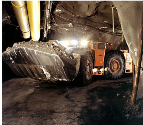
Figure 42. Shows an LHD with its bucket loaded with ore. (Education Material LKAB, 2011)
