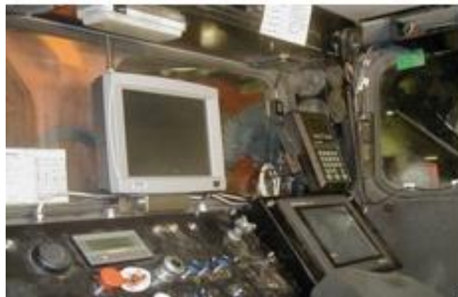
Figure 46. Showing the cabin in a LHD with all screens. (Education Material LKAB, 2011)
