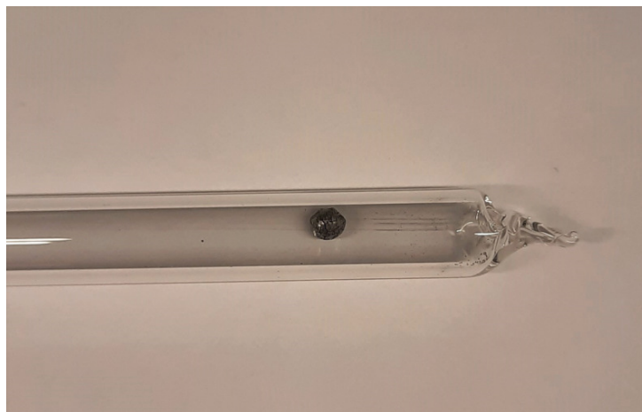
Figure 3.2: A melted ingot of a MnCoSi sample sealed in an evacuated quartz ampoule for the temperature treatment process.
