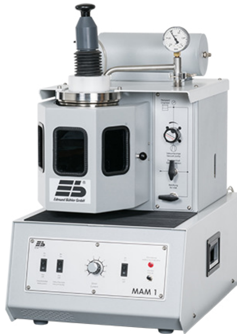
Figure 3.3: Picture of used arc melter model "Mini Arc Melting System MAM-1" from the Edmund Bühler GmbH, taken from [57]. It shows the steering knob on top of the arc melting chamber and the valves for the vacuum system on the right side of the chamber. The lower panel allows to adjust and start the direct current.
