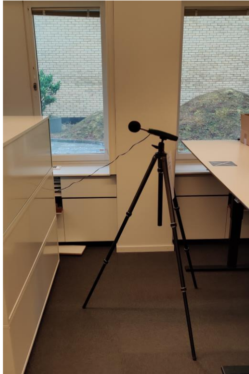
Figure 9. Norsonic 140 placed for measurement at the office on floor 2.
