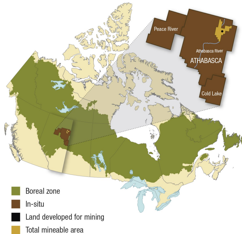
Figure 2. Map showing size of Alberta Tar Sands compared to Canada. The land mass of the three deposits is 142 200 km 2 . The mineable surface available for open-pit mining (yellow) is approximately 4800 km 2 (3.4%) (Government of Alberta, 2021), while the rest is available for in-situ mining (brown) (NRCAN, 2016). This Federal Government created map omits the environmental impact from in-situ mining - the majority of mining conducted - and only shows the impact from open-pit mining (black) (NRCAN, 2016).
