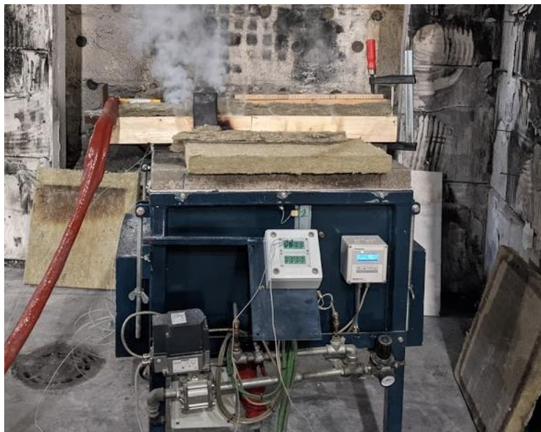
Figure 21. Specimen 1 exposed to the fire curve
