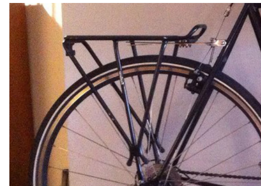
Figure 4-37 - the asymmetrical configuration of a pannier rack (source: flickr.com/photos/wcouch/8675049697)
