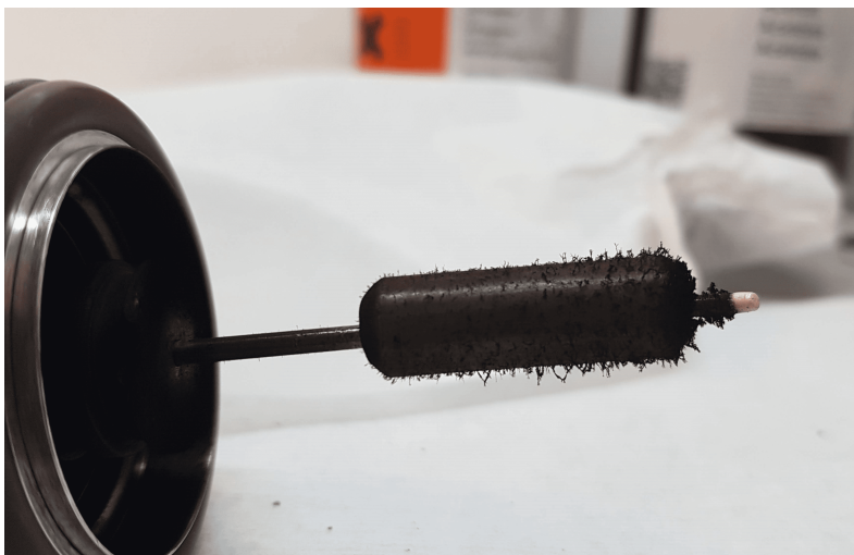
Figure 30: Some particles are not transported away from the chamber with the carrier gas and might get stuck on the electrode or the electrode holder.
