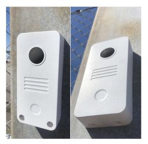
What was concluded from the project was that large conical ports were able to produce the best speech intelligibility in wind. The conical port could be placed both in a front or down facing position, but when placed on the front a wind reducing add-on, as for example a metallic mesh, was recommended.
