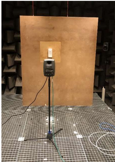
Figure 4.7 Overview of the setup for conducting the Continuous Sweep in the anechoic chamber.
