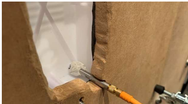
Figure 4.6 The placement of the measurement mic on the back of the prototype.
