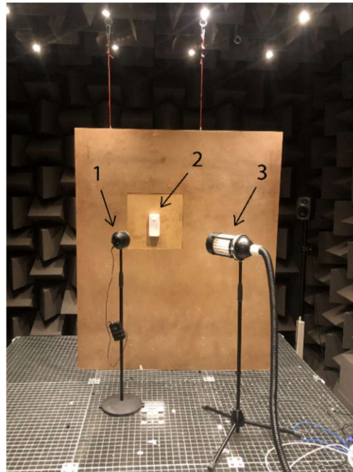
Figure 4.4 Audio recording setup. 1. is the mouth speaker, 2. is the prototype fitted with a microphone and 3. is the air flow generator.
