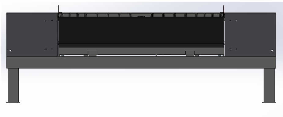
Figure 3.7: Front of 60 kN dock leveler. Note the single main beam.
