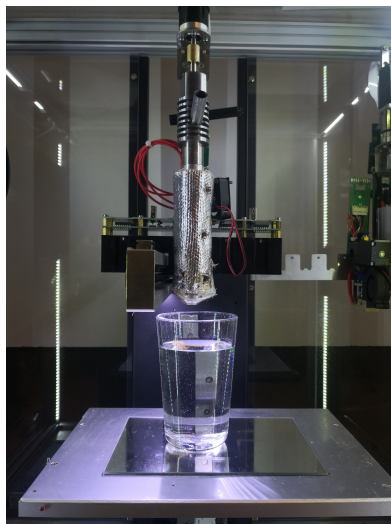
Figure 3.2: Extrusion setup with water bath
