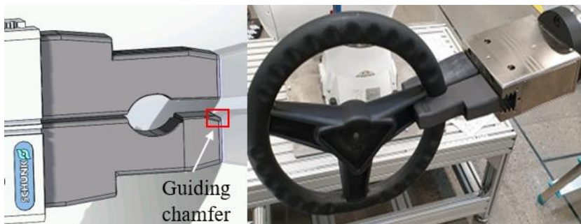
Figure 27. Left: final CAD design of steering wheel fingers, right: 3D printed fingers gripping steering wheel
