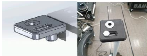
Figure 26. Left: CAD Model of Screw holder, right: 3D printed screw holder that was used in the temporary setup
