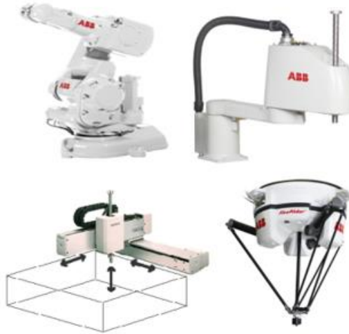
Figure 4. Top left: ABB 140 6-axis articulated arm robot, top right: 4-axis ABB 910 SC Scara robot, bottom left: robot with cartesian configuration, bottom right: ABB IRB 360 FlexPicker, parallel configuration [16], [17],[18],[19]
