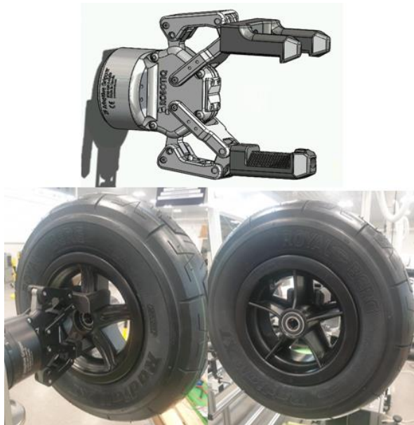
Figure 28. Top: CAD assembly of the front wheel gripper, bottom: the 3D printed fingers gripping the front wheel
