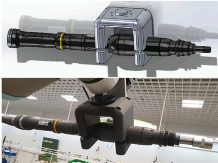
Figure 29. Top: nutrunner ETD-STR61-90-13-T25 , bottom: 3D printed fixture for UR16e
