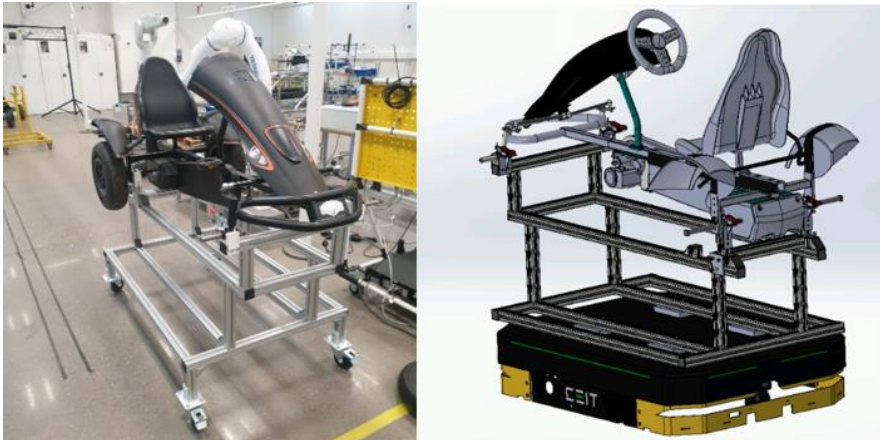
Figure 32. Physical fixture with wheels and CAD fixture design mounted on AGV
