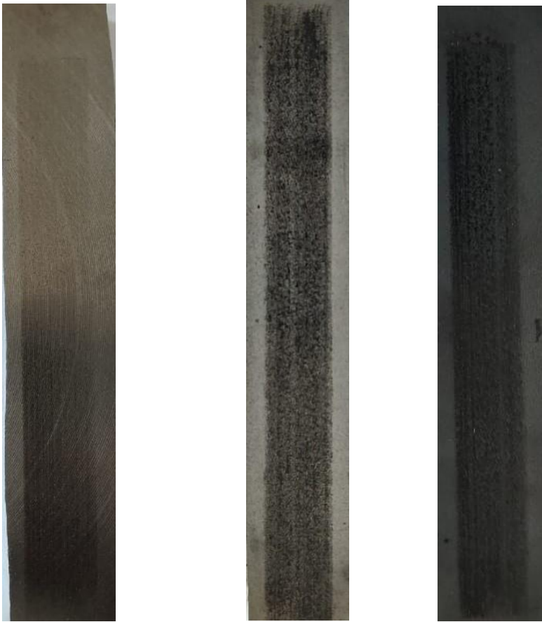
Figure 34: The photograph of the wear tracks of different brake discs for velocity 0.1m/s and 2.5MPa. a) GCI b) FNC and c) Corr-I-Durr discs
