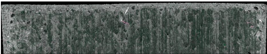
Figure 32: A microscopic view of Tool 3 edge for Velocity 0.1m/s and 2.5MPa for FNC disc
