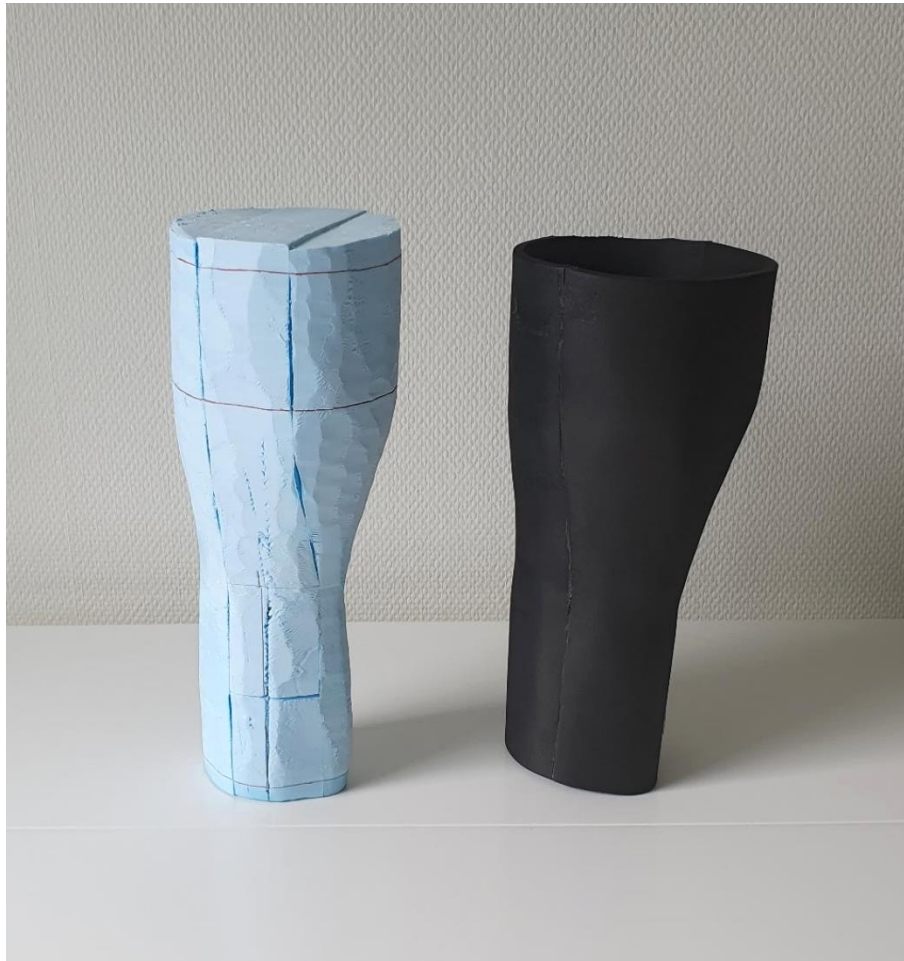
Figure 6.17: The second XPS mould and a prototype in 6 mm EVA foam.
