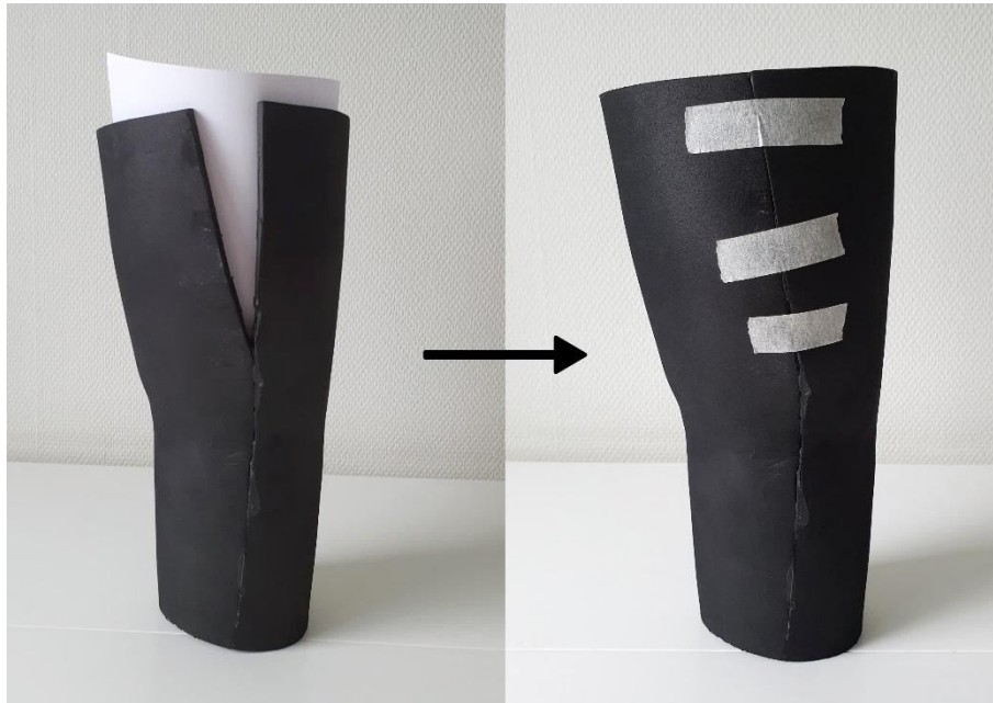
Figure 6.18: A prototype with a V-shaped cut out and the seam that it creates when glued together.
