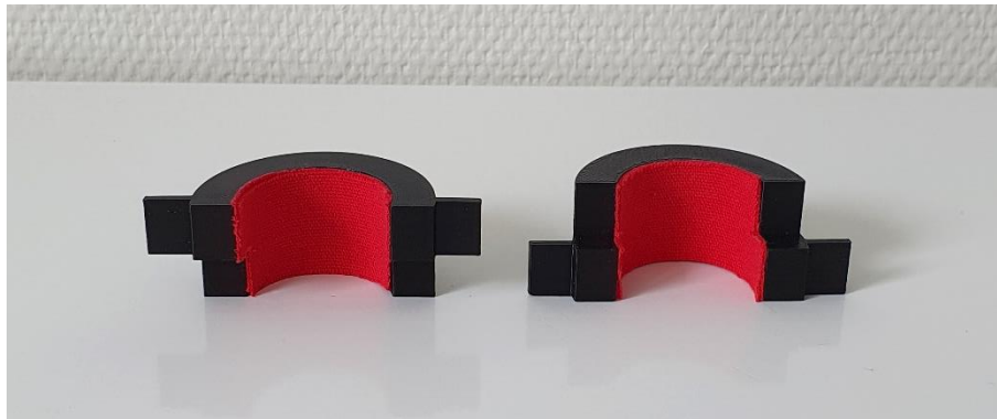
Figure 6.13: Prototype of the second attachment piece with textile tape.
