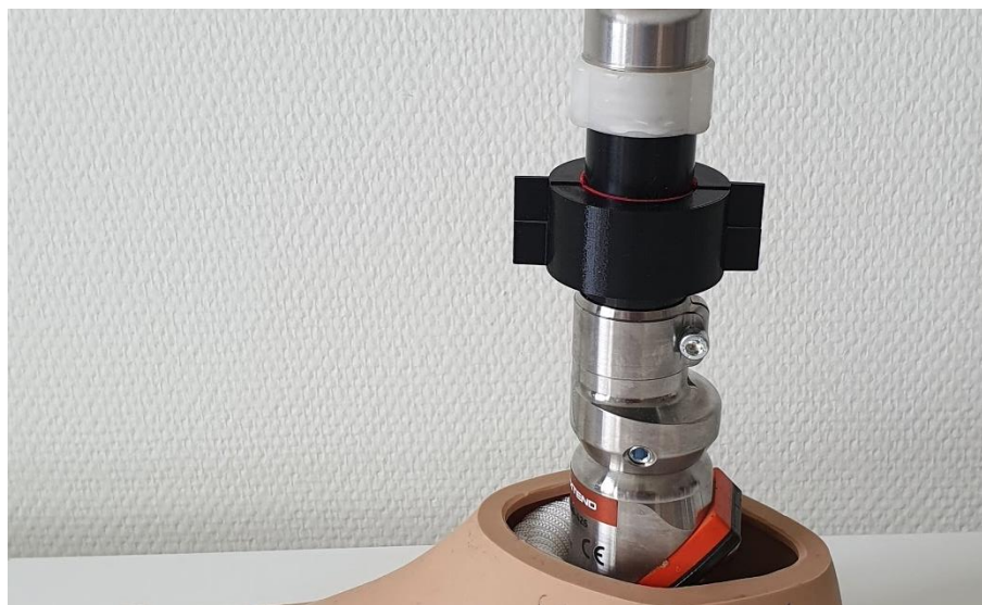
Figure 6.14: The second attachment piece on the pylon.
