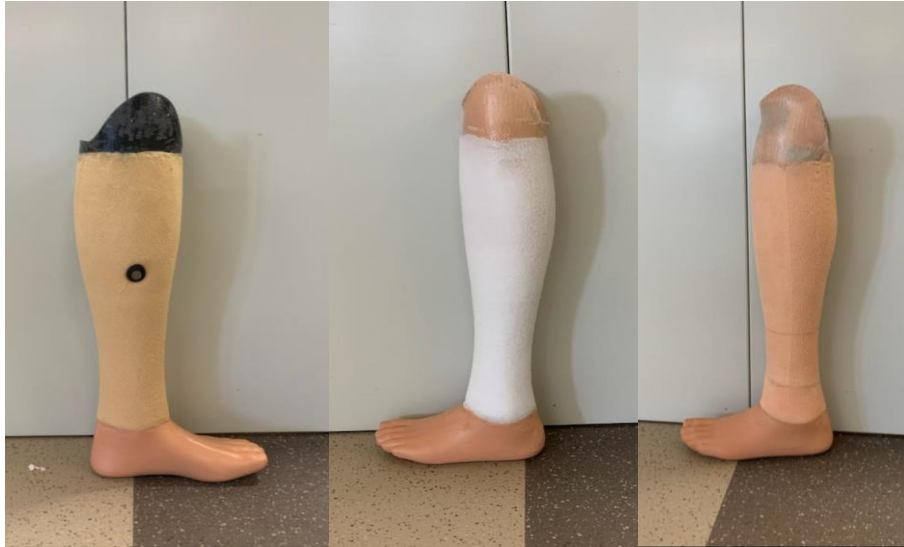
Figure 3.8: Three different foam cosmeses that has been shaped as a lower leg.
