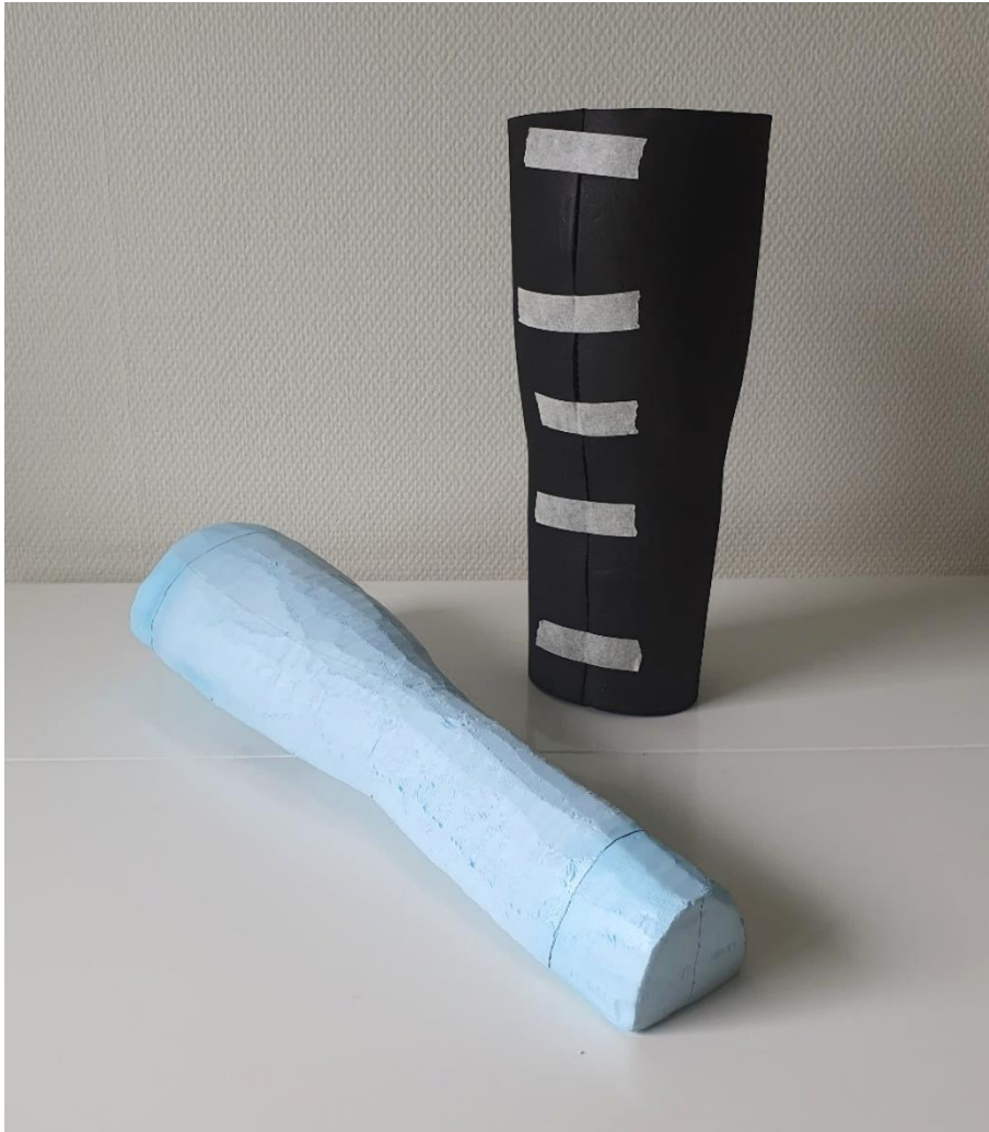
Figure 6.15: The first XPS mould and a prototype in 6 mm EVA foam.
