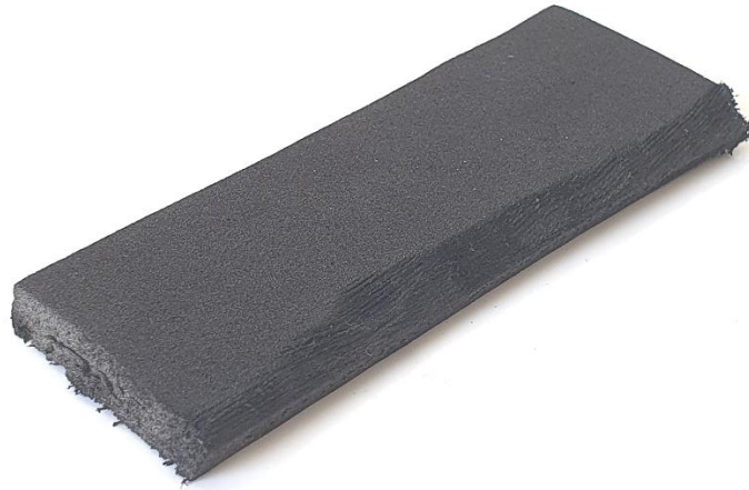
Figure 6.16: A piece of EVA foam where the edge has been sanded down to see if a smoother transition could be obtained.
