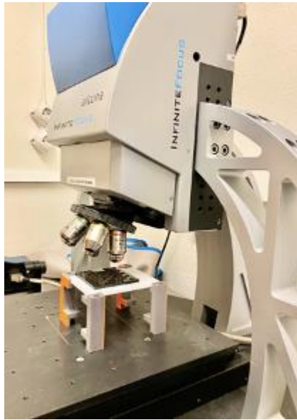
Figure 6. Drilled CFRP panel placed under Alicona
