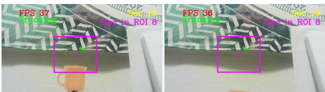
Figure 4. MEDIAN FLOW losing track of the object but keeps bounding box attached to the background.
