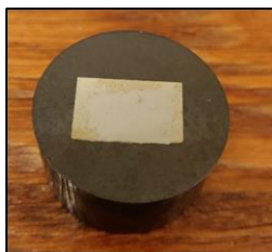
Figure 28 sample embedded in epoxy
