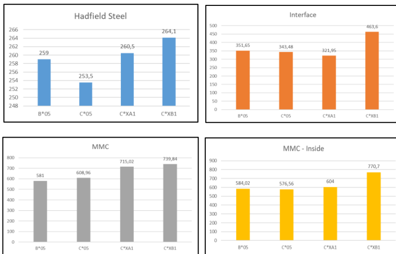
Figure 53 Graphs of average hardness values at different locations (Hadfield steel, Interface, MMC at interface and MMC-inside)
