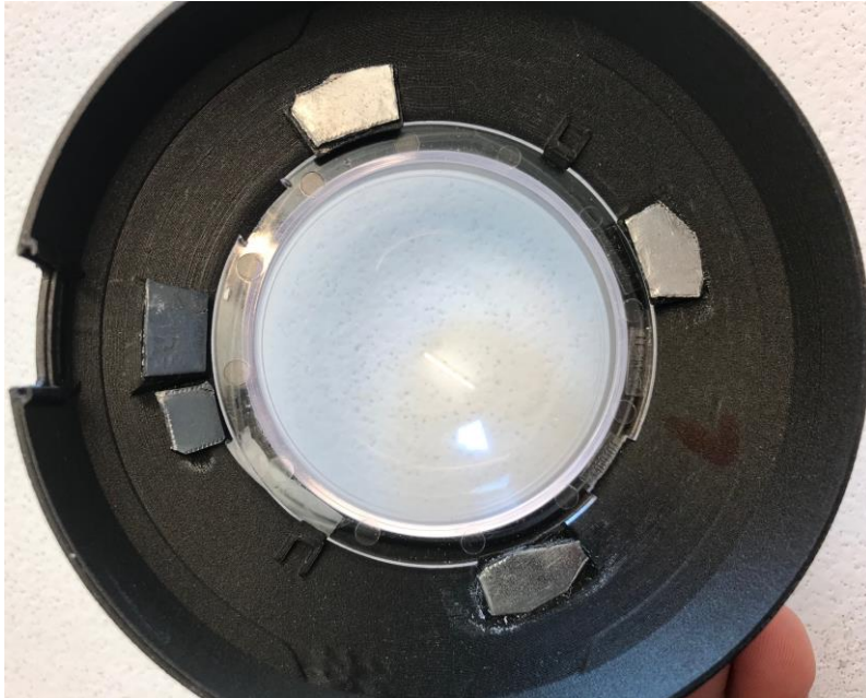
Figure 60 The cover with four cuts of a steel plate glued onto its designated places. (Michael Lindberg)
