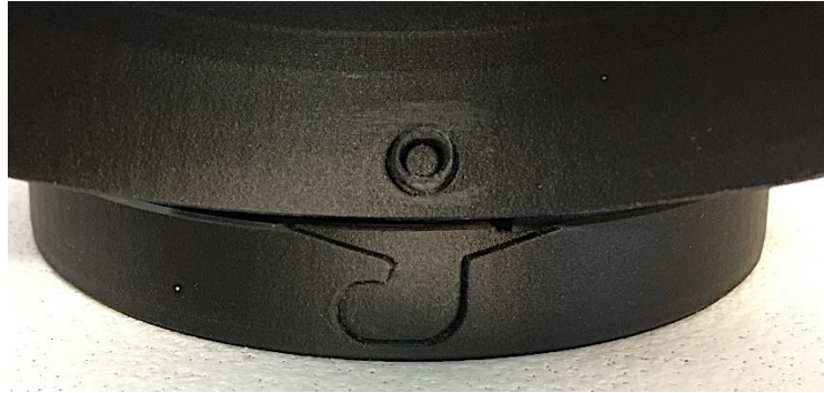
Figure 61 The bayonet prototype, with a circular male protrusion on the inside of the cover and a female trail in the chassis. (Otto Reerslev)
