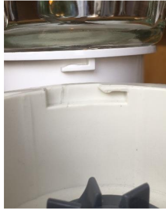
Figure 45 The blender has an L-shaped lock and a corresponding catch, which gives feedback for both locking and unlocking. (Otto Reerslev)
