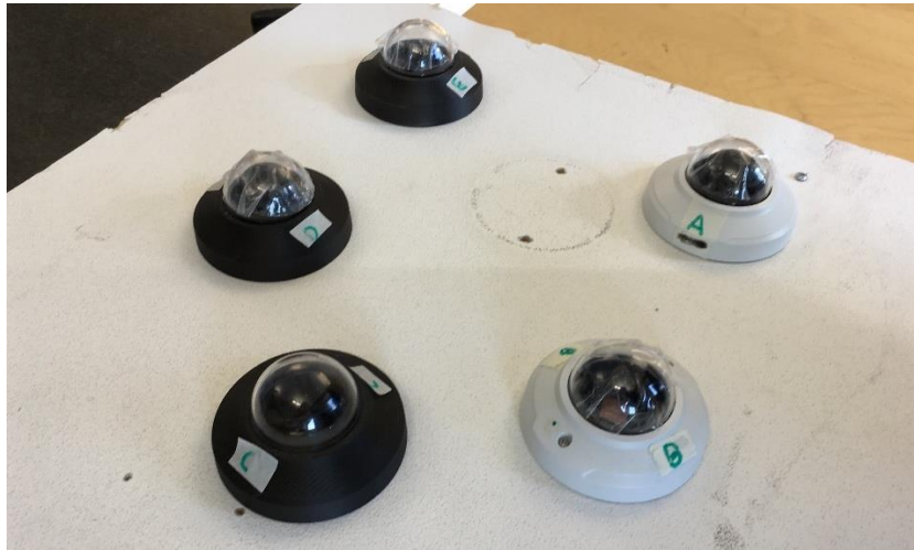
Figure 65 The soft tile before installation in the ceiling, with the three prototypes and the two reference models. Each model was marked with A-E to indicate the order for disassembly, without explaining the underlying concept. (Otto Reerslev)
