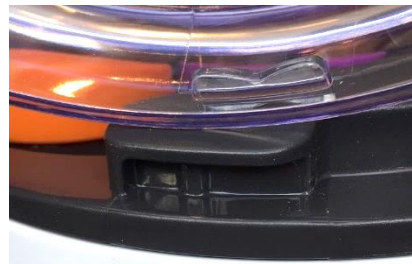
Figure 47 A big food processor with a bayonet lock, where radial catches prevents the container from unlocking. (Otto Reerslev)
