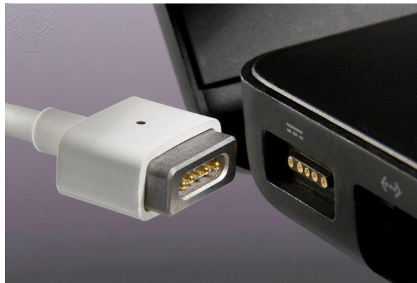
Figure 31 A Magsafe charger held in place by a magnet. (Library)
