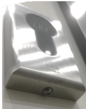
Figure 43 The cover for a wall-mounted RFID-reader is secured with a screw located under the product, out of sight for users. (Otto Reerslev)
