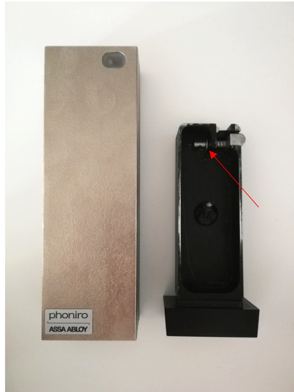
Figure 4.5: The key storage is removed. The red arrow points to the latch that must be pulled to the left in order to remove the key storage.
