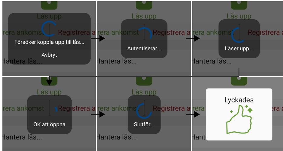
Figure 4.10: Flow chart of the messages displayed on the screen during the unlocking process.
