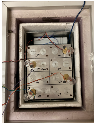
Figure 19 Loaded calorimeter with pressure sensors connected.
