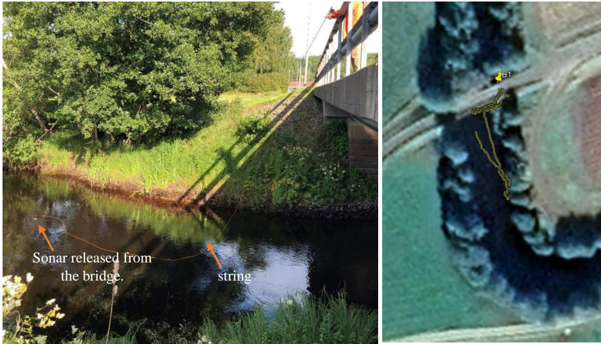
Figure 9 (Left) Bathymetric measurement of river from deep sonar method. (Right) Measured points (yellow dots in the figure) from the sonar measurement near the B1.
