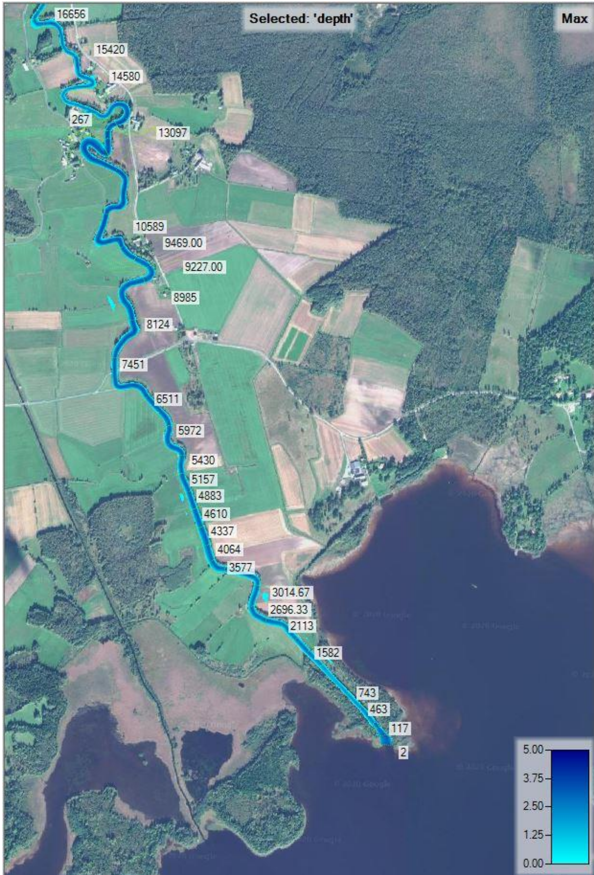
Figure B. 5 Depth mapping for simulation result for maximum water surface profile for year 2004-2019 (5/5)
