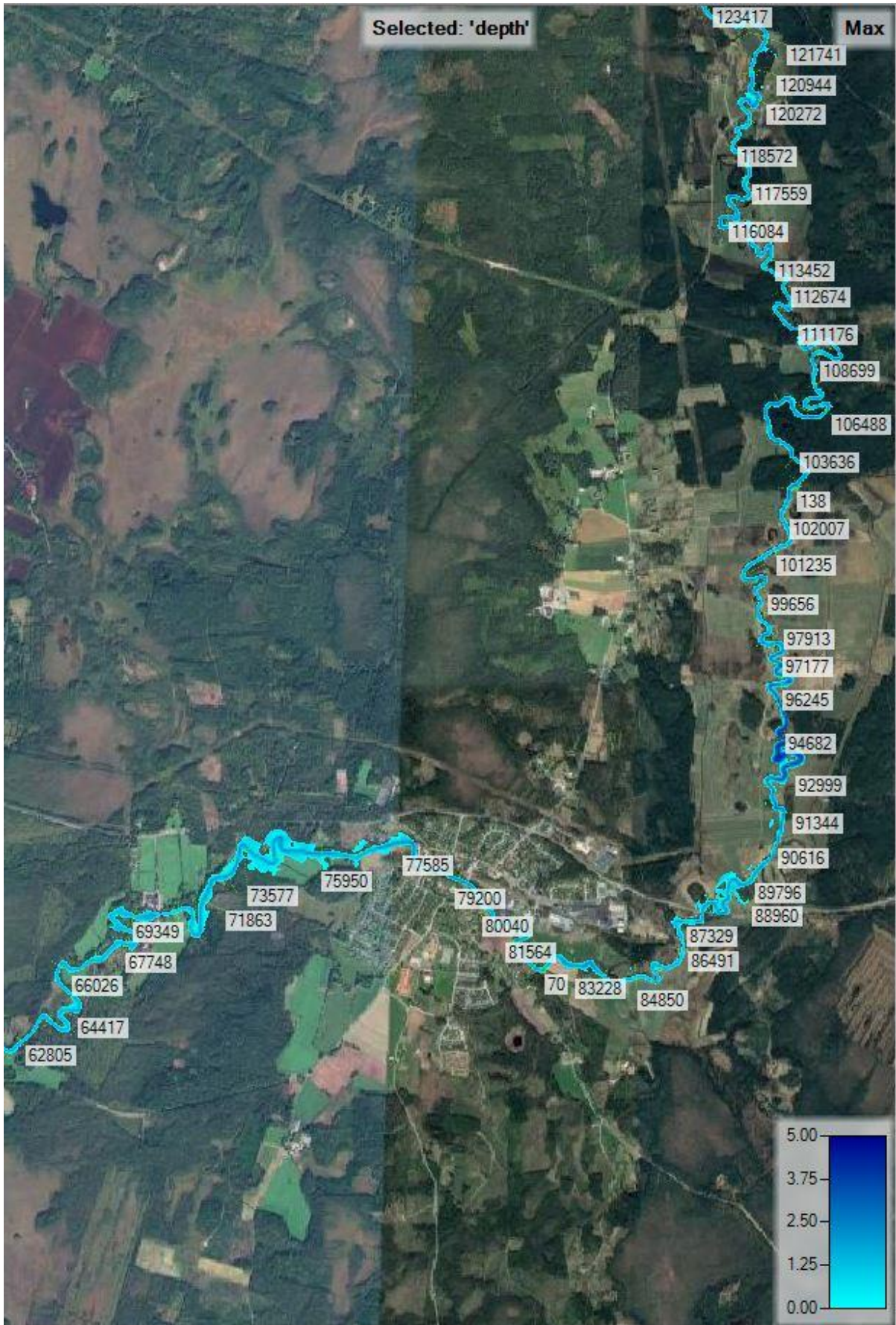
Figure B. 3 Depth mapping for simulation result for maximum water surface profile for year 2004-2019 (3/5)
