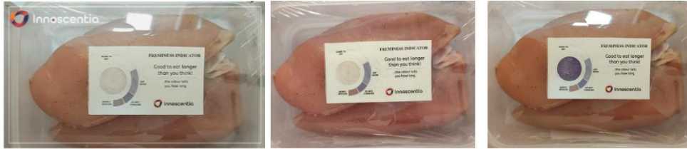
Figure 4. Illustration of sensor colour change as an indicator of meat freshness
