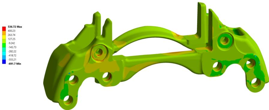
*Figure 68: Carrier Test 2 - Maximum Principal Stress Distribution*
