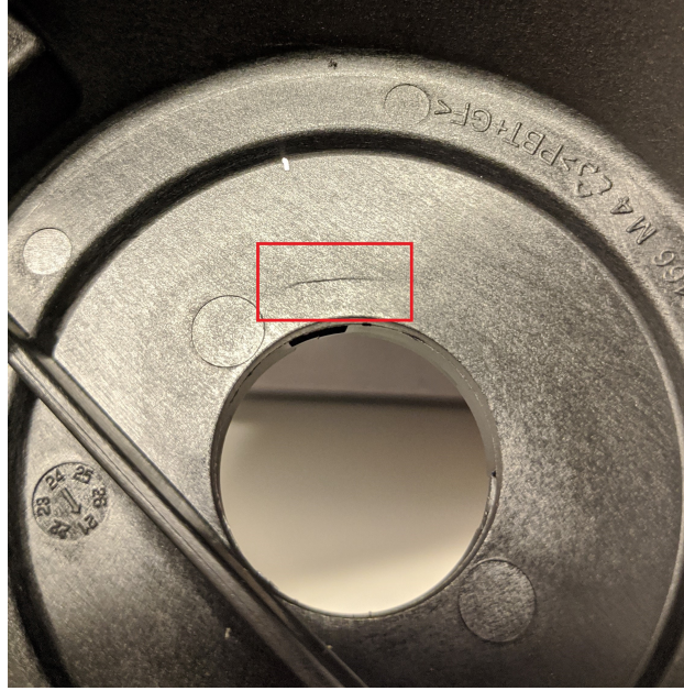
Figure 22: The crack in part (A), which appeared after the first impact test IK 8 on recycled plastic.
