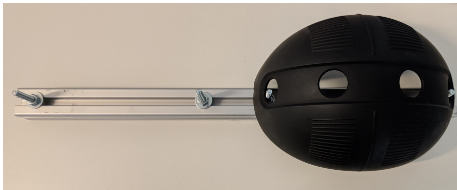
Figure 12: The mount upon which part (D) was mounted for inducing stresses during the organic oil test. The distance between screws was the same for all samples.
