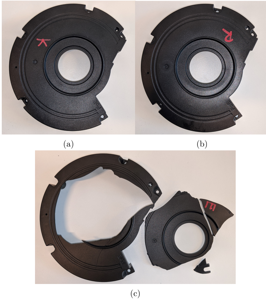
Figure 17: Part (E) in the three plastics after being submitted to a compression test. (a) is the conventional plastic Cycloy, (b) is the recycled plastic Infino, and (c) is the biobased plastic EcoPaXX. The conventional and recycled plastics showed some indentation from the probe, and the biobased plastic suffered from a brittle failure.
