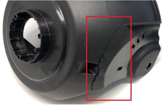
Figure 41: The crack of part (A) after one compression test on a subassembly.
