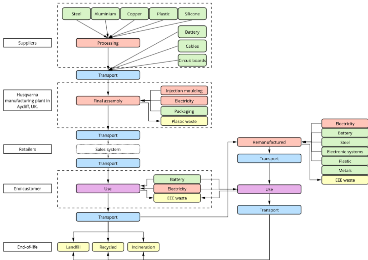
Figure 4. Process flowchart of the robotic lawn mower AM550, cradle-to-grave, with the remanufacturing process. Processes with dashed lines are excluded from the analysis.
