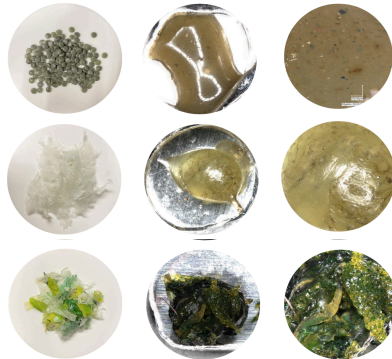
Figure 4. 2 An example of separated films used in DSC analysis. Top to bottom: recycled granules, Fraction 1 (colorless), Fraction 9 (green); left to right: before DSC, after DSC, close-up after DSC
