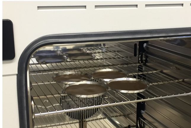
Figure 3. 6 All 12 samples placed in the oven; placement on the top rack avoids strong convection that may disturb the samples
