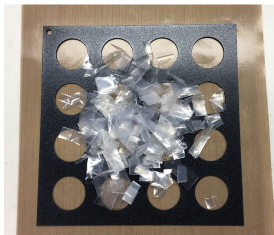
Figure 3. 5 Cut sample on Teflon form and Teflon sheet ready to be covered and formed into discs
