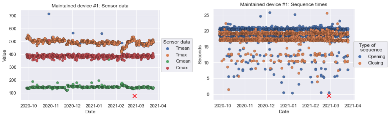
Figure 6.33: Device measurements before and after reset: Group 1
