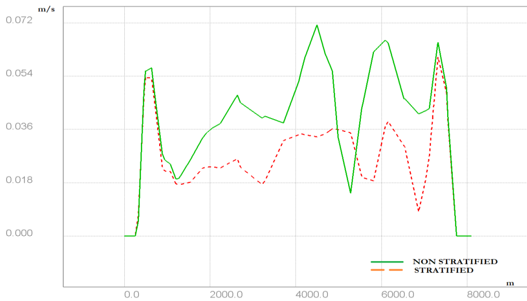
Figure 7-17 Steady State scalar velocity distribution in cross section D for stratified and non-stratified condition
