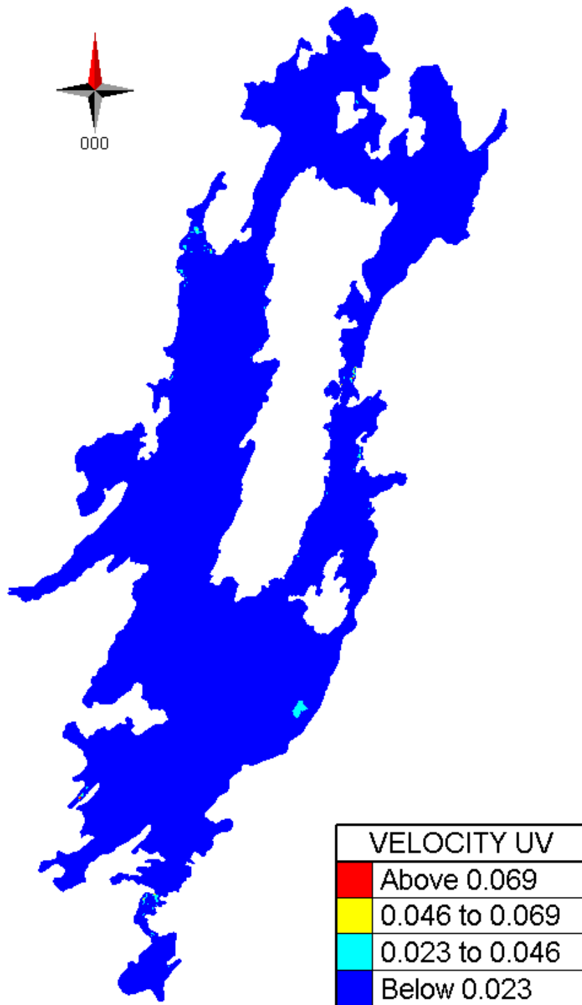
Figure A 24 Contour Scalar Velocity distribution (uv) for wind 2.5\text{ms}^{-1} from southwest Direction
