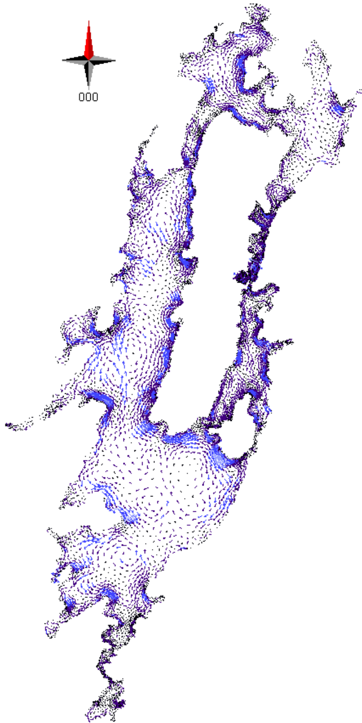
Figure A 13 Lake current patterns observed for simulating 10\text{ms}^{-1} wind from NorthWest
