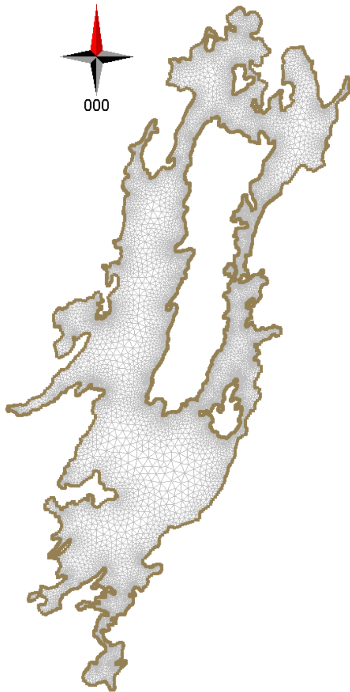
Figure A 4 Defining the no flow boundaries(non permeable) and liquid boundaries in the mesh , Blue Kenue
