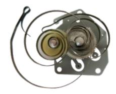
Mechanical kitchen timers use clockwork to measure time, which includes gears, springs, an escapement and a pendulum or a balance wheel. These parts work together to ensure the proper operation of the timer.
