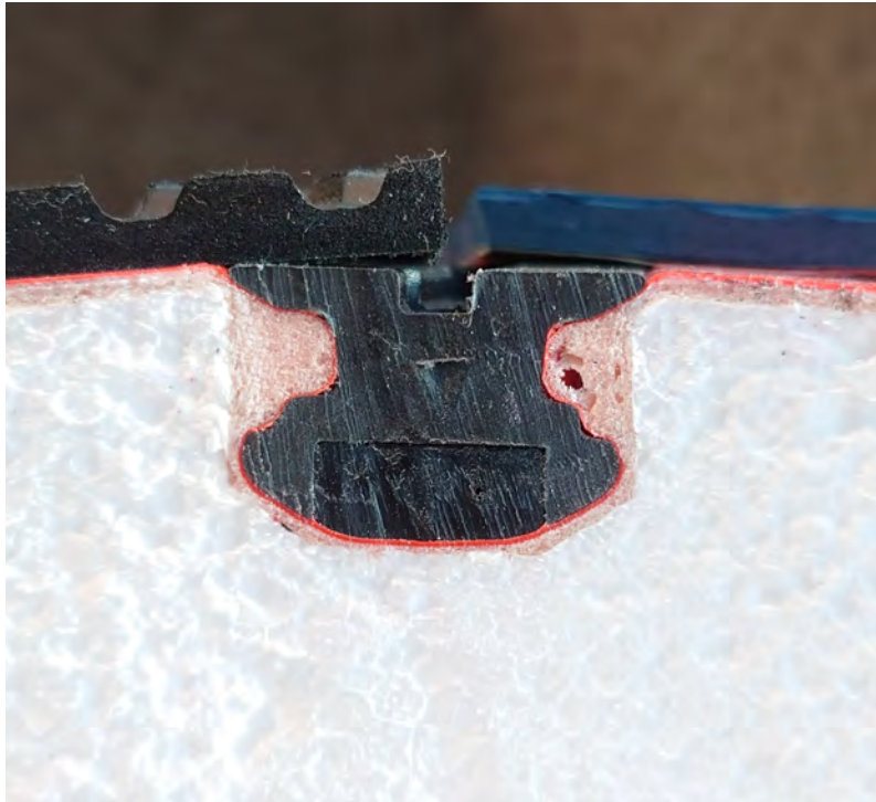
Figure 4.2: Example of capture moulding.
