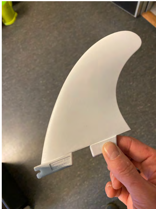
Figure M1: The fin needed to be spray-painted before scanning.
