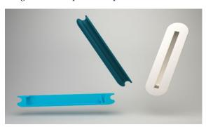
The fin plug concept allows for different assembly methods of a jetboard and consists of a simple geometry design. A design which allows for easy manufacturing, maintenance and dimensioning. The concept was chosen through user testing of 3D printed prototypes. In the tests, this concept excelled through its auditive feedback and firm grip. Above all, it enabled the producing of jetboard optimised fins
