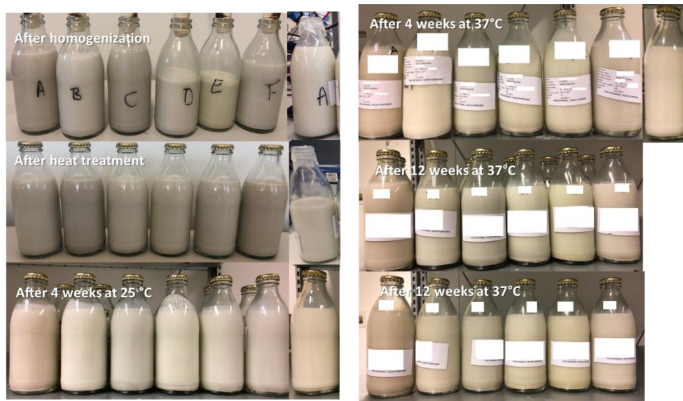
Figure 1 Visual assessment of the samples. Samples from left to the right; 1.0, 1.2, 1.4, 1.5, 1.6, 1.7, and 2.0.
