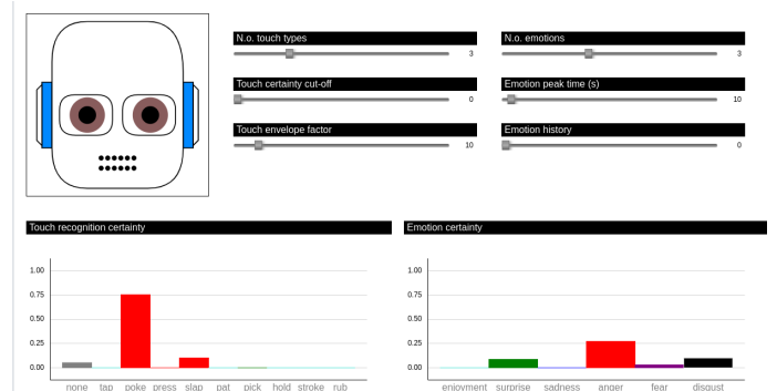
Figure 11: Screenshot from Ikaros WebUI for displaying an Epi response to touch. Parameters are set to select three touch types (slider in the upper middle). Primarily a poke, secondarily a slap, is detected and a none touch for background is also identified (lower left bar graph). An emotional response of anger, disgust and surprise, in that order of magnitude of strength, is produced (lower right bar graph). An expression of red-brown colour is produced by the merging of related colours in the eyes of the Epi head (above left).
