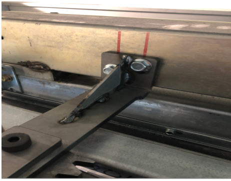
Figure 5.3: Triangle added to the wall mount.
