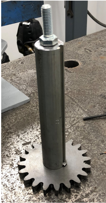
Figure 5.7: The shaft extension.
