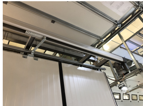
Figure 3.4: The current drive system at ASSA ABLOY.
