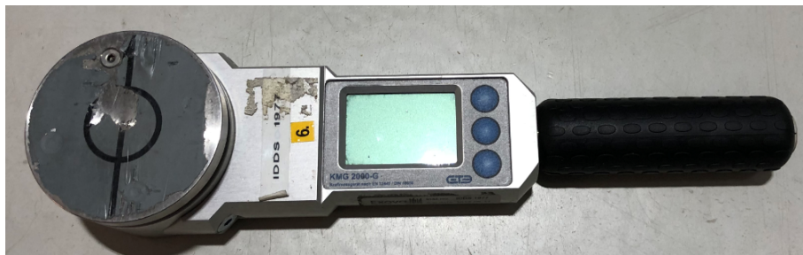
Figure 2.7: Image of a measuring device designed specifically for the EN 12453 test.
