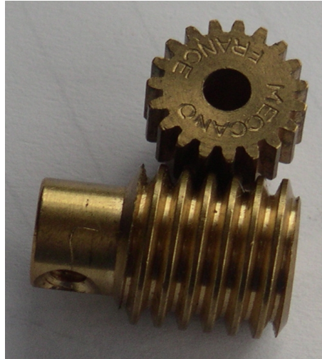
Figure 2.14: Worm gear set. Figure from [9]. Public domain.
