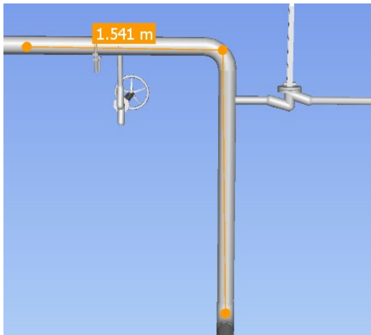
Figure 3.12: Measuring tool in Naviswork Freedom 2019.
