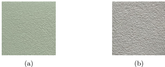
Figure 12: Images of the spray coated samples where a) flame sprayed and b) plasma sprayed sample from University West. The colors of the plates are, as seen in the figure, greenish-grey and grey respectively.
